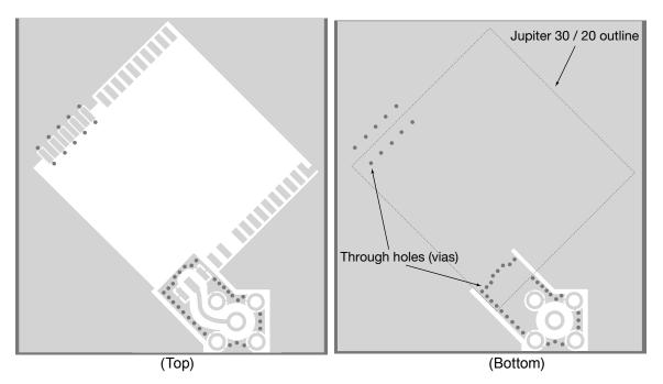
Figure 2-5: Example PCB layout for external active antenna
