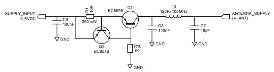
Figure 2-9: Simple current limiter circuit
