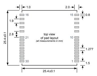
Figure 2-3: Recommended application layout dimensions
